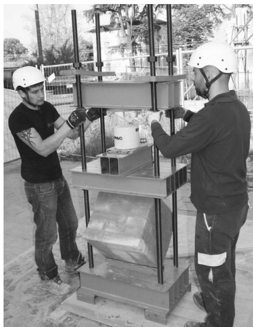
Figure 7. Setting of the loading machine for shear test through diagonal compression.
