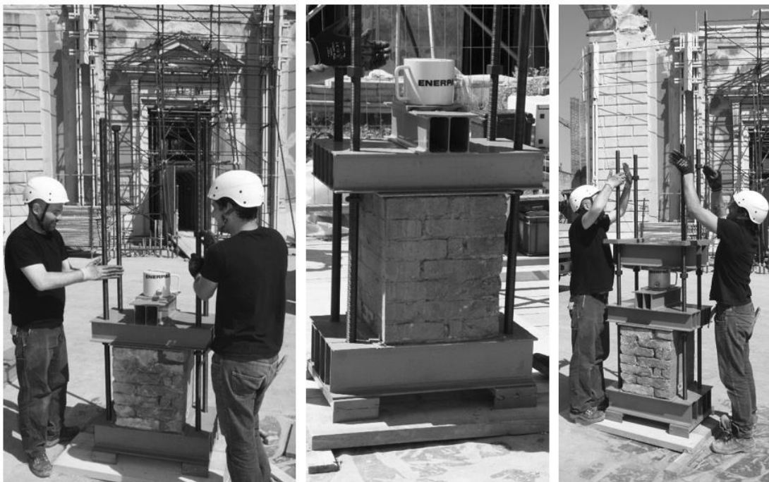
Figure 6. Phases of installation of the loading machine for compression test.
