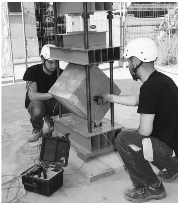
Figure 10. Measure of the sonic velocity in several points of the masonry sample.
