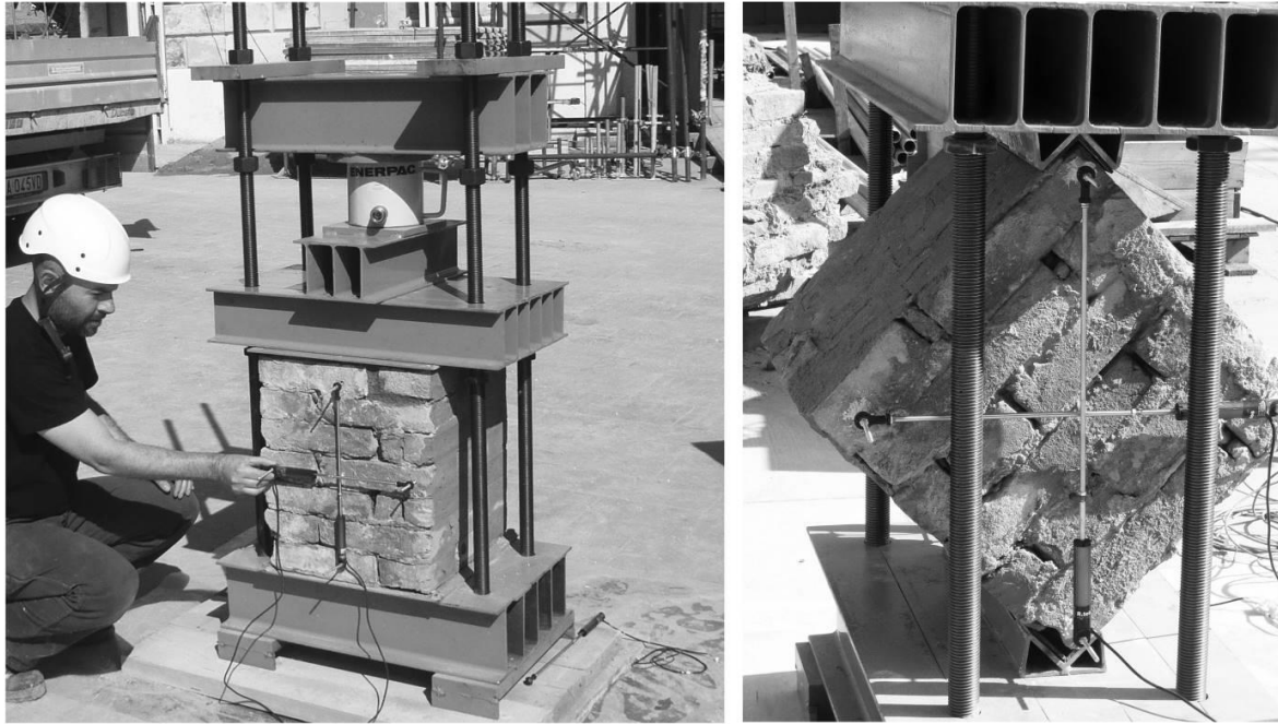
Figure 9. The deformations of the masonry specimens during compression and shear tests are measured by electrical transducers connected to an automatic acquisition system.
