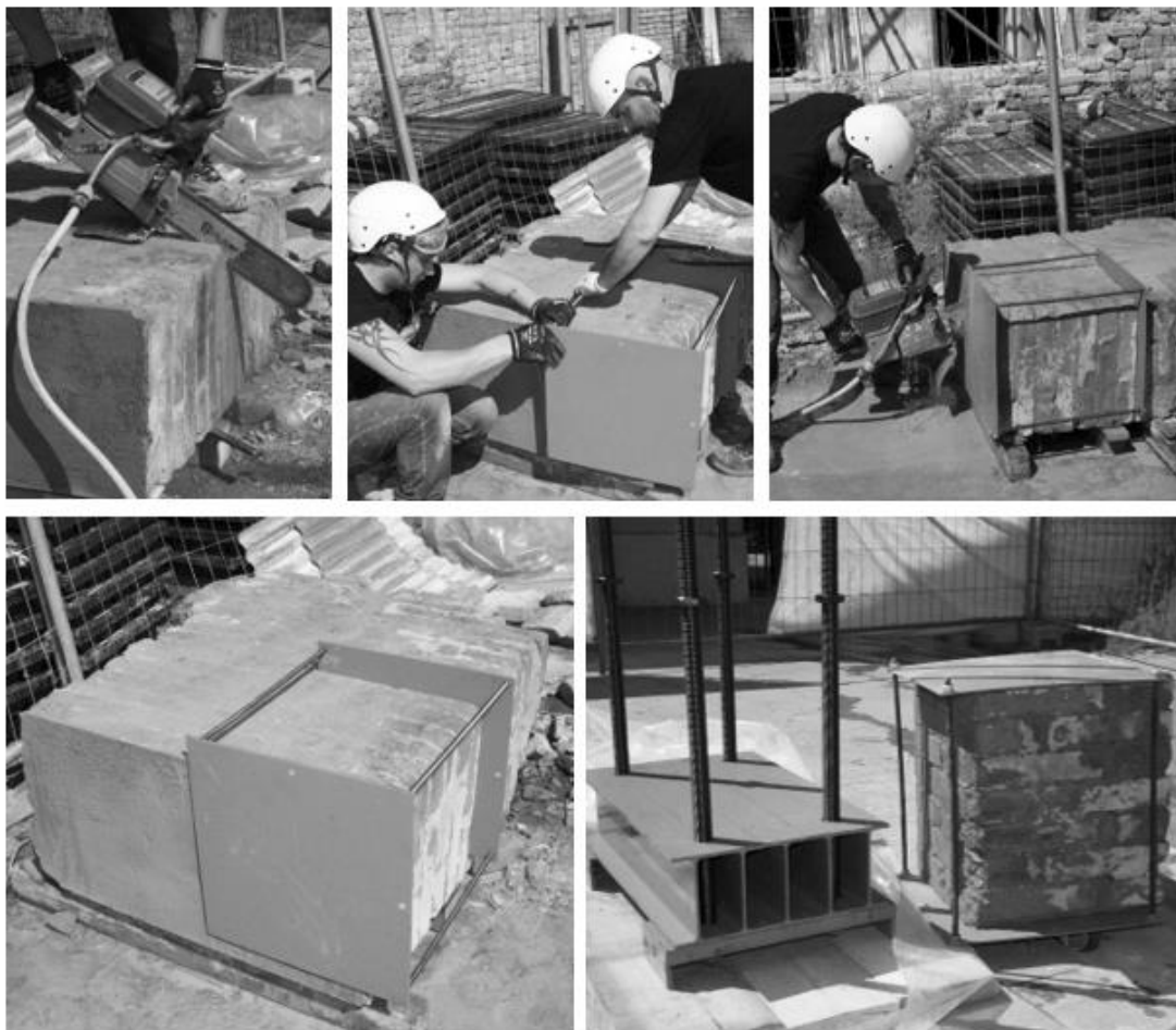
Figure 4. Cutting of the large size masonry specimens for the compression and shear tests. The steel frame used in the cutting phase is shown.
