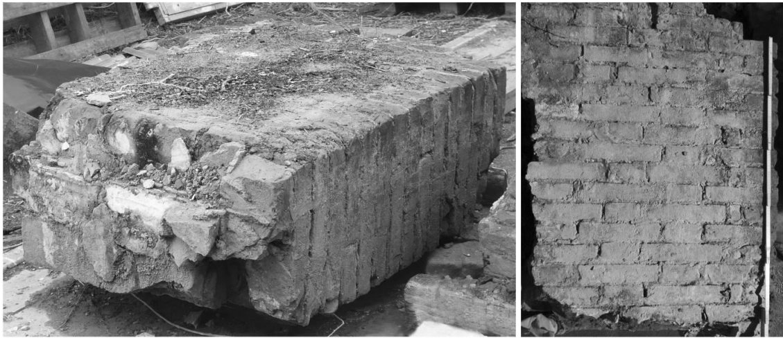
Figure 3. View of the masonry block collapsed during the earthquake and used for the compression and shear tests.
