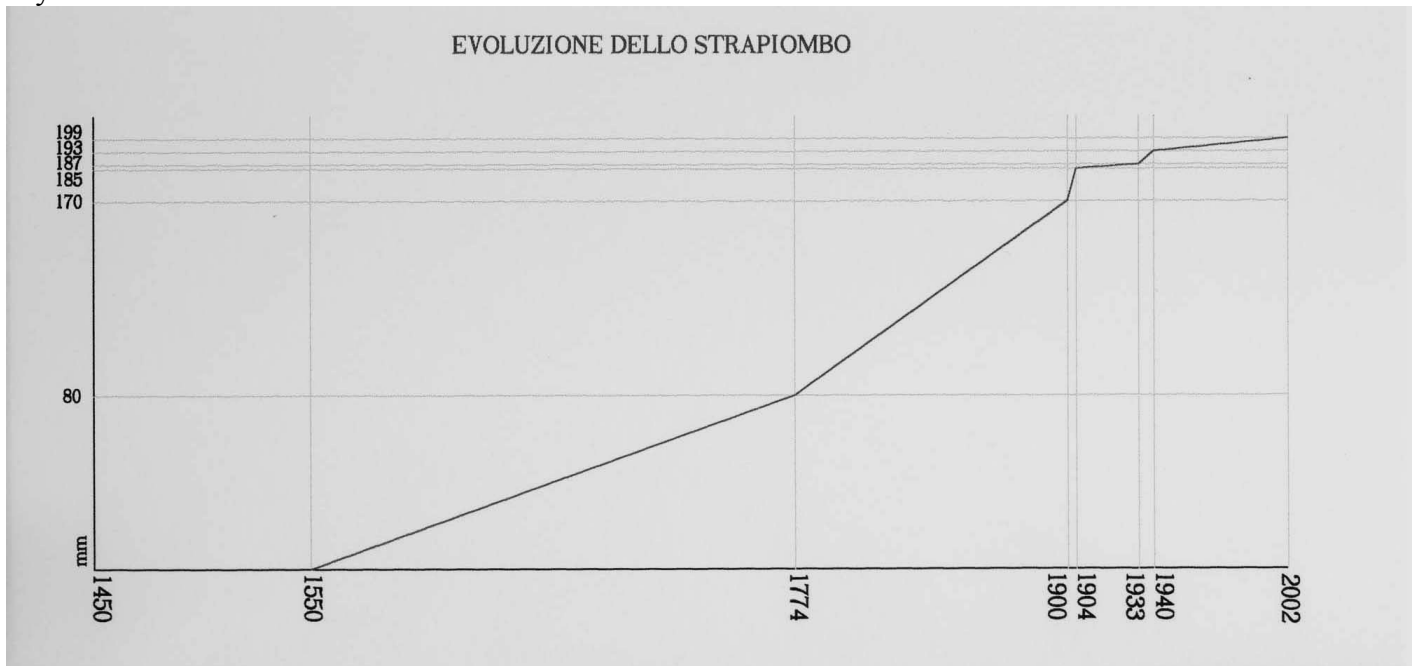
Figure 1. History of the leaning of St Stefano's bell-tower measured at the level of bell's cell (44 m)
